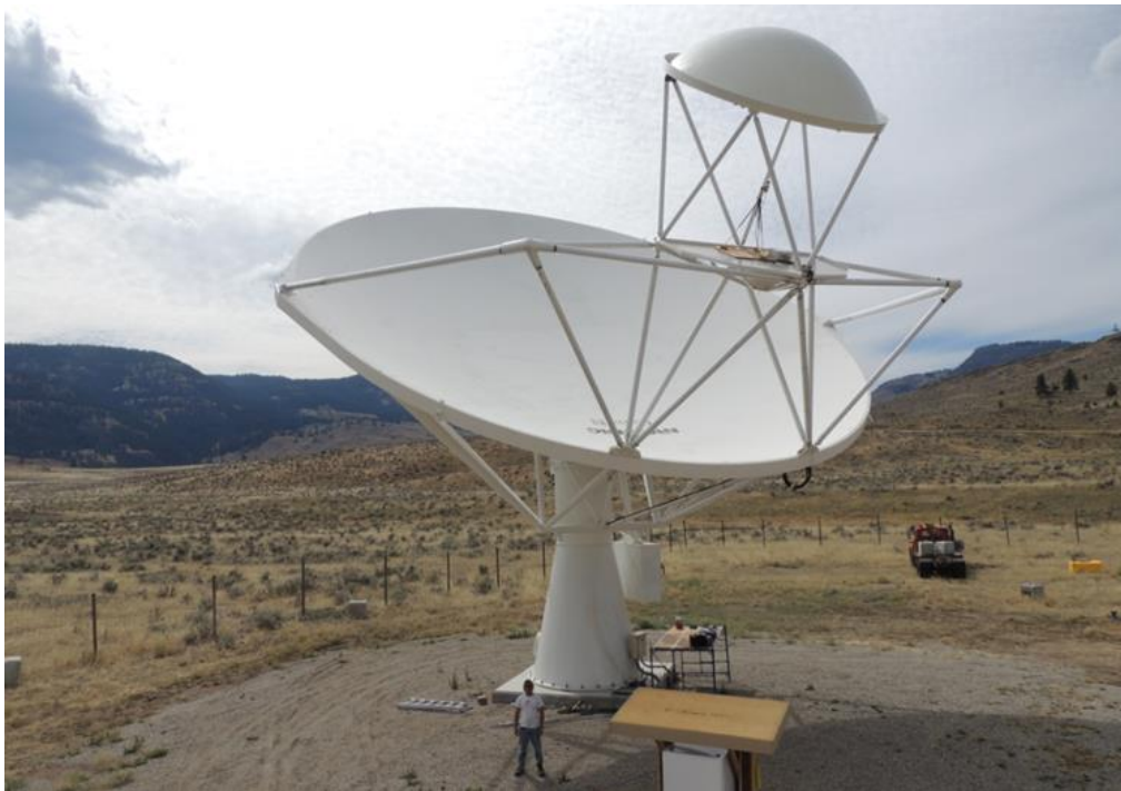
Figure 1. Two views of the Dish Verification Antenna #1 (DVA1) at NRC-DRAO, a novel 15-m diameter, rim-supported composite reflector. This high performance, low cost design is being advanced by Canada to the SKA DISH consortium as part of the SKA Pre-Construction design work.
