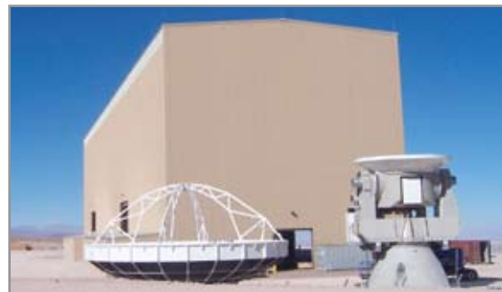
The first production antenna under assembly at the mid-level facility (image courtesy of NRAO).
