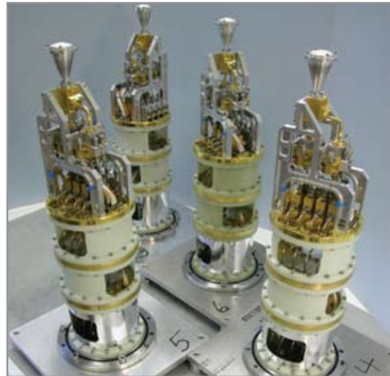
Band 3 cartridges at the National Research Council's Herzberg Institute of Astrophysics (image courtesy of HIA).
