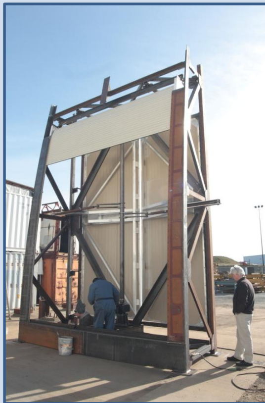
Figure 9 - The full-scale TMT enclosure ventilation module prototype, built by Dynamic Structures Ltd in Port Coquitlam, BC.
