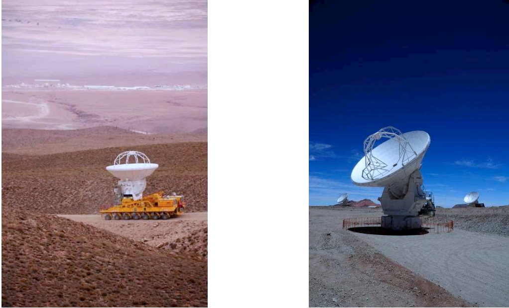
FIG. 3.— (left) Picture of first antenna on its way up to the high site. (right) Three ALMA antennas at the high site, where phase closure was achieved in December 2009. Picture credits ALMA (ESO/NAOJ/NRAO).
